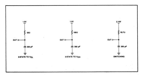
Figure 5. Output Test Load Circuits
